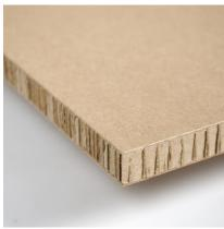
The closed cell design makes Xanita board significantly stronger than visually similar honeycomb board products.
